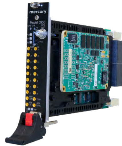
Figure 8 Model 5950 S0SA 3U VPX Quartz Board (cover removed to show QuartzXM Module)
