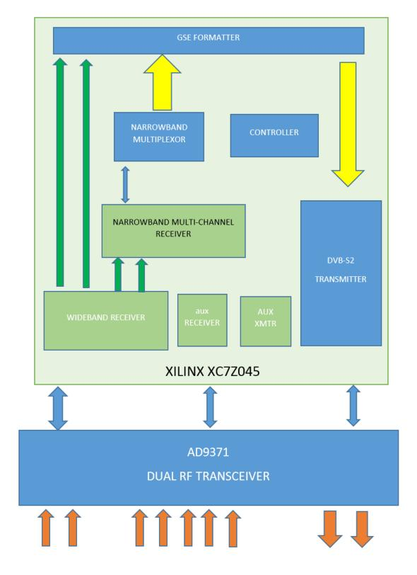
RF connections will include 2 Main Tx, 2 main Rx, and 5 auxiliary RF inputs any one of which can be selected as an additional receiver. These all operate from 300
