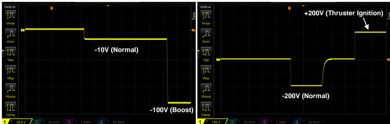
Figure 20. QM HV Aux board test results: cathode bias modes (left) and thruster Accel grid modes (right).
