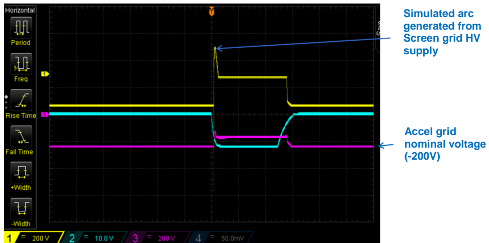
Figure 21. QM HV Aux board test result showing arc-protection on Accel grid supply.
