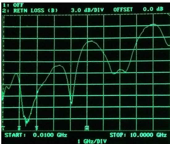
S11 Input (left) & S22 Output (right) Return Loss vs. Frequency 10 MHz to 10 GHz 1 GHz/div. Vertical scale is 3 dB/div. Dashed line at top is 0 dB
