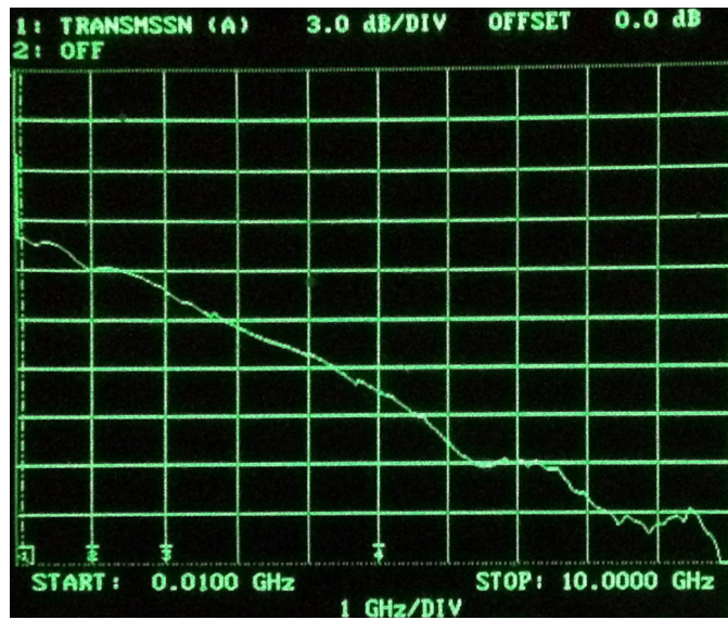
S21 Gain vs. Frequency 10 MHz to 10 GHz, 1 GHz/div. Vertical scale is 3 dB/div. Dashed line at bottom is 0 dB. Useful Gain up to 5 GHz
