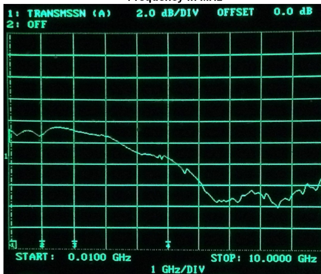
S21 Gain vs. Frequency 10 MHz to 10 GHz, 1 GHz/div. Vertical scale is 2 dB/div. Dashed line at bottom is 0 dB. Useful Gain up to beyond 10 GHz
