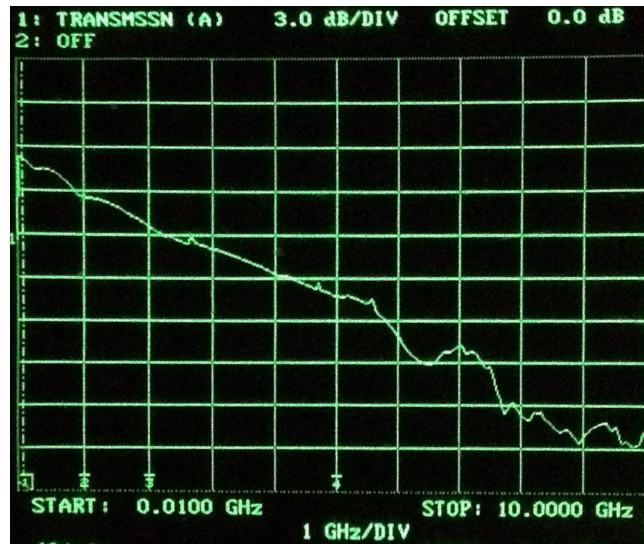
S21 Gain vs. Frequency 10 MHz to 10 GHz, 1 GHz/div. Vertical scale is 3 dB/div. Dashed line at bottom is 0 dB. Useful Gain up to 7 GHz
