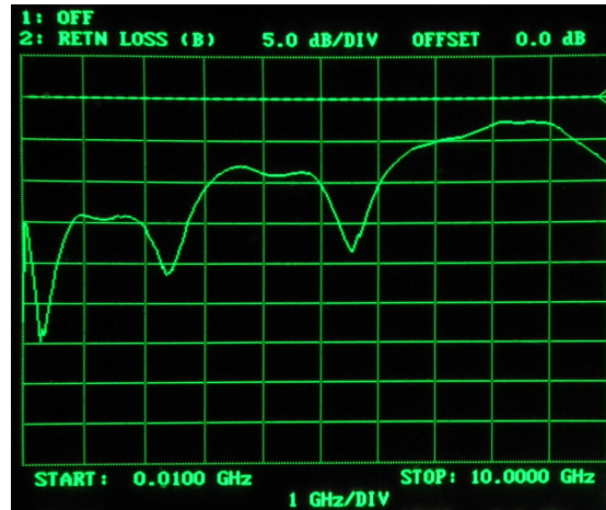
S11 Input (left) & S22 Output (right) Return Loss vs. Frequency 10 MHz to 10 GHz 1 GHz/div. Vertical scale is 5 dB/div. Dashed line is 0 dB
