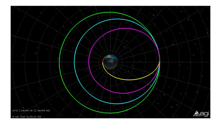
Green is GEO. Teal is feasible for final transit using Busek thruster. This is above the most intense part of the outer Van Allen belts.
