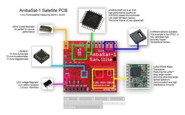
AmbaSat-1 is tiny space satellite kit that you assemble and code yourself. Once your satellite kit is assembled and programmed, it will be launched onboard a commercial rocket which will deploy your satellite into Low Earth Orbit, where it will spend up to 3 months in space.
